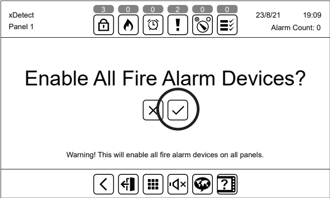
Figure 233. Enabling all fire alarm devices
