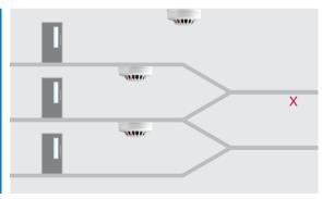
Enclosed stairways should have a detector on the top of the stairway and on each main landing.
