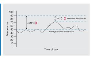
The minimum static response to heat devices should not be less than 29°C above the average ambient temperature, or less than 4°C above the highest temperature the device can be expected to experience.
