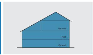
Less than 300m² can be covered by a single zone. When the total floor area exceeds 300m², each floor would require a zone (or zones if the floor area exceeds 2000m²). Stairwells, Liftwells or similar should be separate zones.
