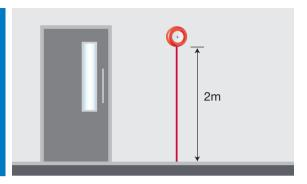
Unless MICC or armoured cable to BS7846 standard is used, consideration should be given to the protection against physical damage from floor level to the height of 2m. Except in relatively benign areas, such as shops, offices and similar, where cabling can be clipped to robust walls.
