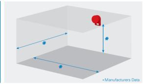
Open class devices do not conform to either the Wall or Ceiling category. However, they still need to meet the required illumination of 0.4 lux over their specified range.
