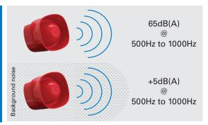
The minimum sound level of a sounder device should be *65dB(A)* or *5dB(A)* above a background noise that lasts more than 30 seconds and not less than 75dB(A) at the beadhead if required to rouse people from sleep. The maximum sound level should not exceed *120dB(A)*.
