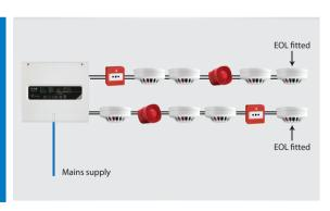
To comply with the current version of the BS 5839 Part 1, the use of fire resistant cables is required for all critical circuits, this includes detection, sounders and mains supply.
