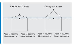
For ceilings that feature an apex: As long as the height of the apex from the rest of the ceiling is less than 150mm for heat detectors or less than 600mm for smoke detectors, then these can be treated the same as flat ceilings. For higher apexes, a device should be installed at the highest point. The coverage of the device in the apex can be increased by 1% per degree of angle of the roof up to a maximum of 25%.
