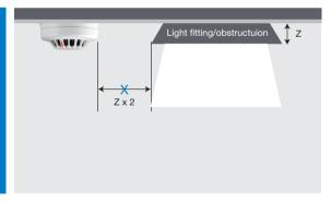
For obstructions less than 250mm deep never mount devices closer than twice the depth of light fittings or other obstructions on the ceiling.
