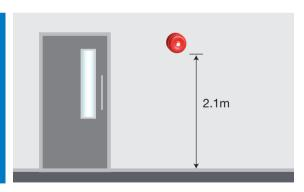
Visual alarms such as beacons should always be mounted at a minimum height of 2.1m from floor level, in a position that is likely to attract attention.
