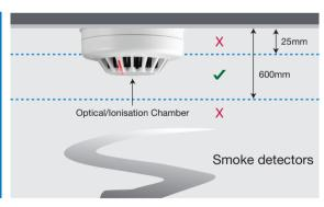
The sensing element of a smoke detection device (optical smoke chamber) should not be less than 25mm below the ceiling, and not greater than 600mm below the ceiling.
