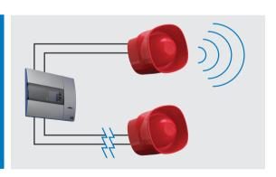
Sounder device cabling should be arranged so that in the event of a fault at least one sounder located within the vicinity of the control and indicating panel will remain in operation.
