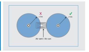
Do not site detectors less than 1m from air inlets or air circulating systems.
