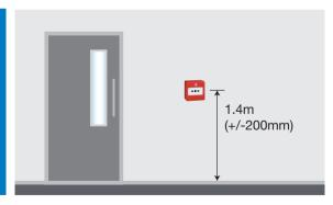
The centre of the element of the manual callpoint should be positioned 1.4m (+/-200mm) from floor level (unless a wheelchair user is likely to be the first person to raise the alarm, when this is applicable it should be noted on any certification). All manual call points should be fitted with a protective cover, which is moved to gain access to the frangible element.
