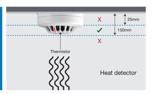
The sensing element of a heat detection device should not be less than 25mm below the ceiling, and not greater than 150mm below the ceiling.
