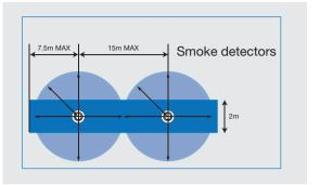
In corridors less than 2m wide the horizontal spacing of detectors can be increased, the area of coverage need not overlap as in the case of a room. Any corridor over 2m wide is deemed to be a room. Coverage should be provided as appropriate to system category.
