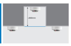
Voids less than 800mm in height are required to have a risk assessment to determine if AFD is required. Voids in excess of 800mm require independent coverage.
