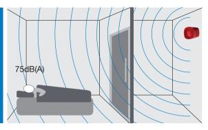
For areas where people are sleeping, sounder devices should produce a minimum 75dB(A) at the bed-head with all doors shut. In buildings likely to provide sleeping accommodation for the hearing impaired, consideration should be given to the incorporation of both audio and visual devices.
