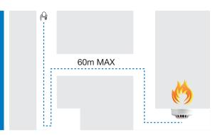
The maximum zone floor area should not exceed 2000m². A person searching a zone for a fire should not have to travel more than 60m from the zone entrance to identify the source of the fire.
