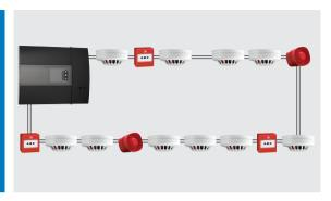
On a loop system, short circuit isolators are required to limit the effect of one fault to less than 2000m<sup>2</sup> floor area. Two simultaneous faults on a circuit should not disable protection within an area greater than 10,000m<sup>2</sup>.
