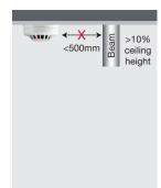
A device should not be mounted within 500mm of any obstruction. If the top of a solid partition is less than 300mm from the ceiling then it should be treated as a wall. Similary, ceiling obstructions such as beams should be treated as walls if deeper than 10% of the ceiling height (particularly important in voids).
