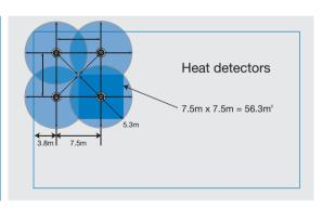
When mounted on a flat ceiling, heat detection devices have an individual coverage of 5.3m radius. However these radii must overlap to ensure there are no 'blind spots'. Therefore individual coverage can be represented by a square measuring  $7.5\times7.5m$  giving an actual coverage area of  $56.3m^2$  per device.
