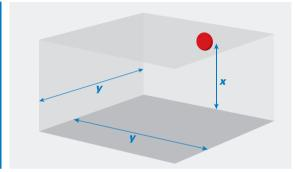
x – The maximum height of the device on the wall in metres, with a minimum value of 2.4m
